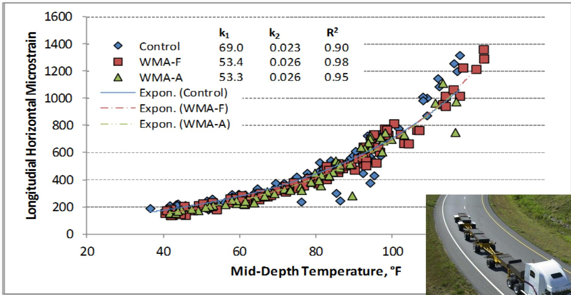
No Statistical Difference between WMA and HMA sections
