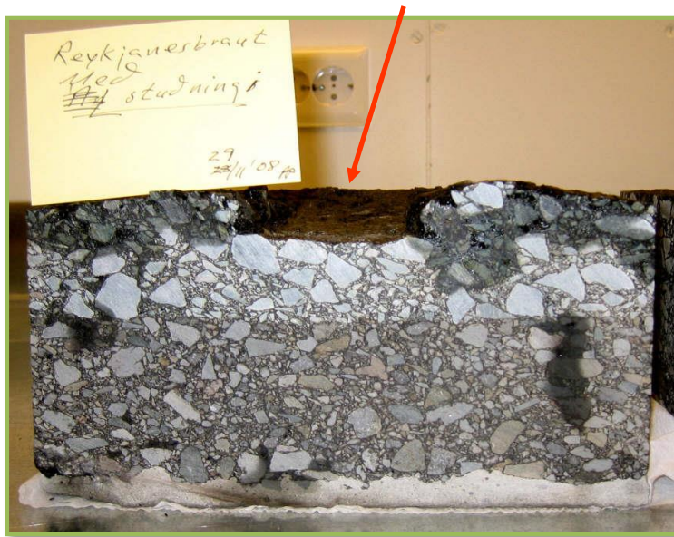
Rut depth 12,2 mm, tested at 45°C
