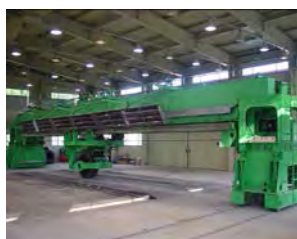
Figure 1. Rutting Evaluation of LEADCAP WMA using APT Test Facility
