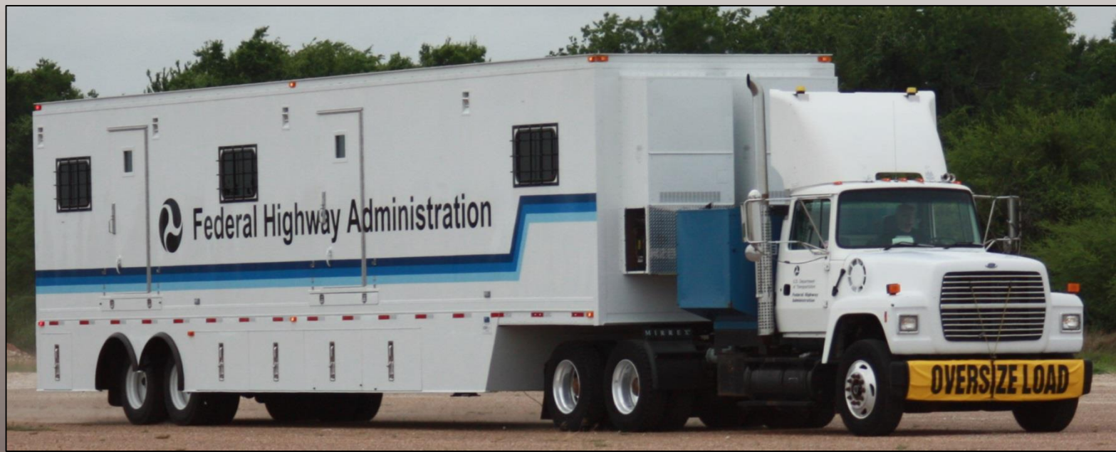
FHWA's Mobile Asphalt Testing Trailer – “the MATT”
